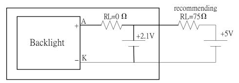
b. E/L B/L driven from A.K cable directly
