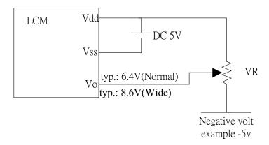
\*(Option) LCM operating on "DC 3V" input with external negative voltage
